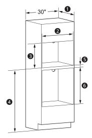
If you are replacing an electric double oven with the combined installation of a wall oven and a speed oven, use the dimensions shown. The middle rail separating the two openings may need to be larger than the 2" minimum shown.
