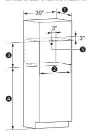
Order a 30" wide single oven cabinet or cut the opening in a wall to the dimensions shown.
