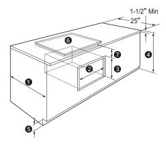
Gas or electric cooktops may be installed over this oven. See cooktop installation instructions for the cutout size. This oven requires a separate, properly grounded 16-Amp, 120-Volt, 60Hz power supply. The cooktop requires a separate power supply. Use a 36" or wider base cabinet.
